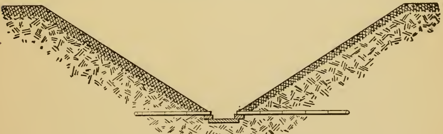
Fig. 2—CROSS SECTION OF DITCH
